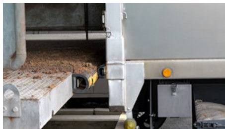
There is no height difference between the loading ramp and the cargo bed.
