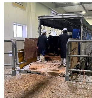
(Installation of side panels to prevent falls)
